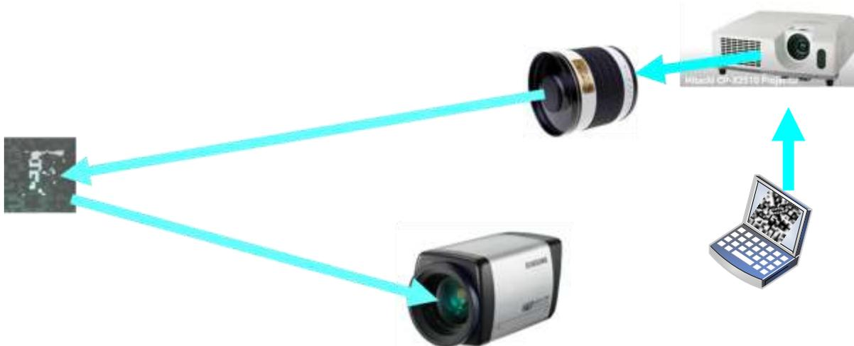
**Figure 2.** The single-pixel imaging arrangement in the visible area
