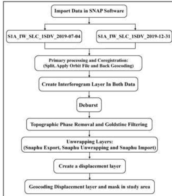
**Figure 1.** Innovative method: Flowchart of Dinsar data processing
